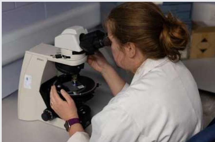
Figure 6-8: Image of a PCM being used by a laboratory analyst
