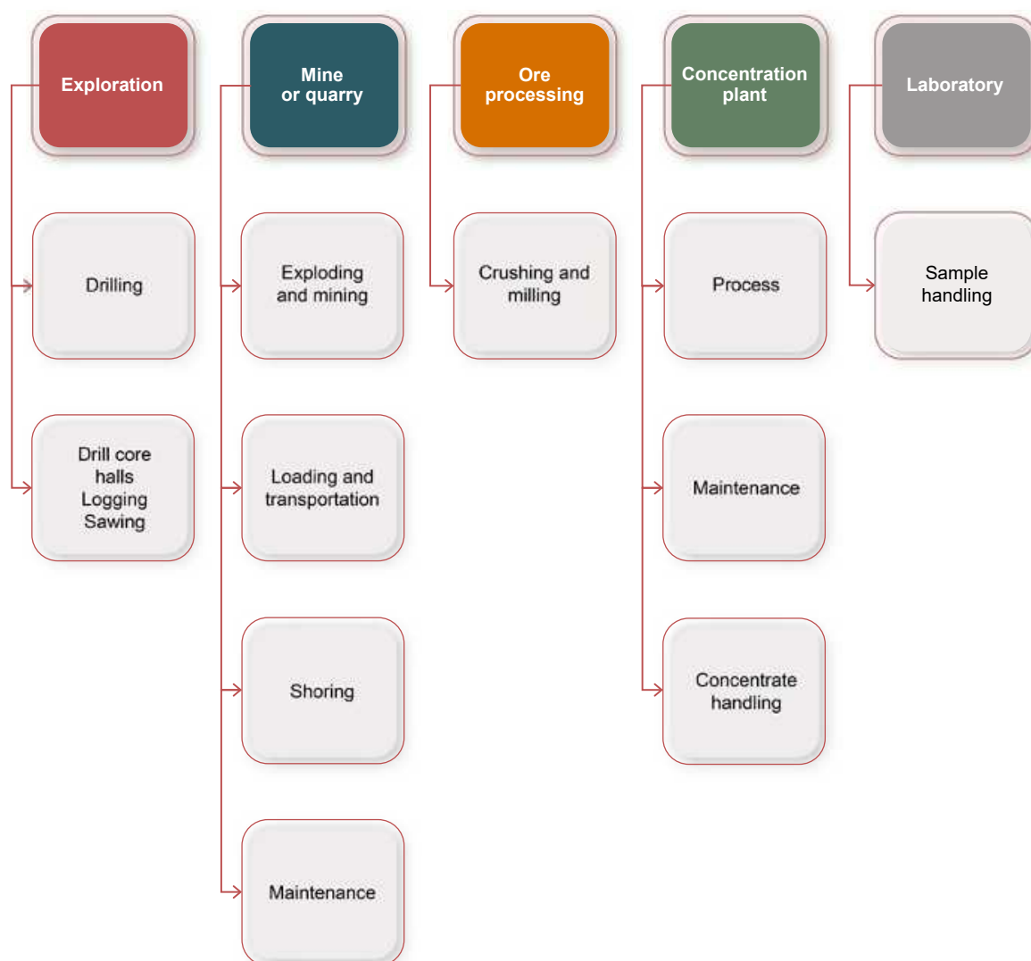
Figure 15-2: Division of mining or quarrying operations into measurement compartments and areas
