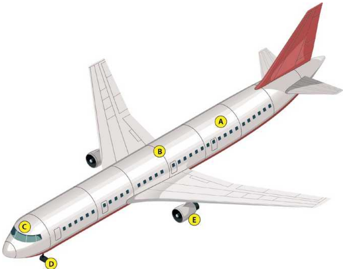
Figure 14-5: Aircraft – where asbestos might be found (non-exhaustive)
