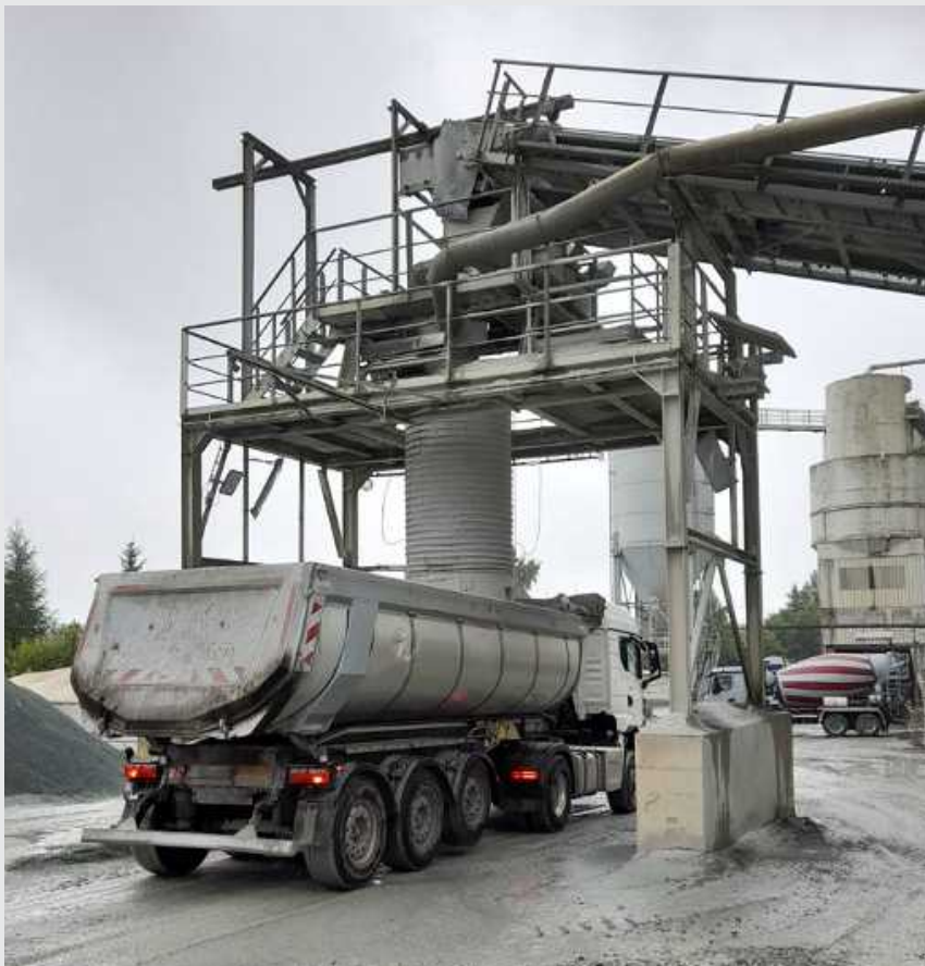
Figure 15-5: Height-adjustable truck-loading spout with dustproof skirt
