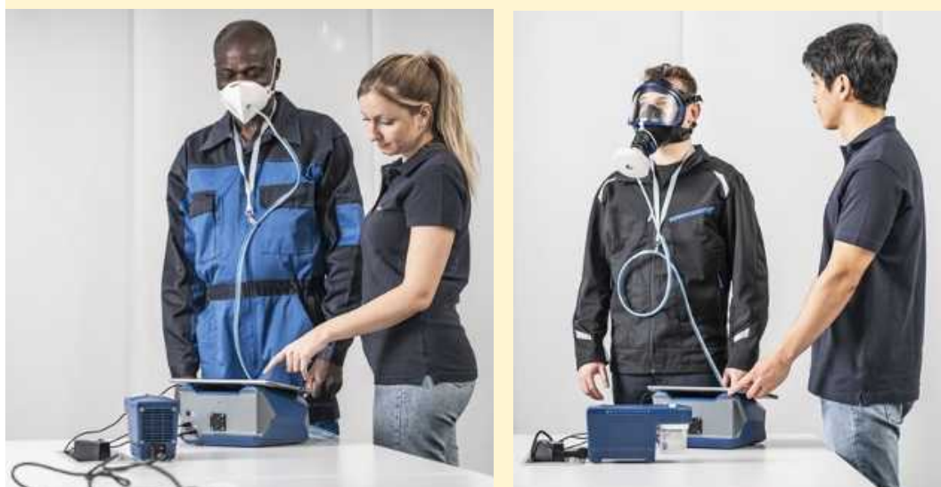
Figure 8-12: Examples of face-fit testing for full face mask and filtering facepiece
