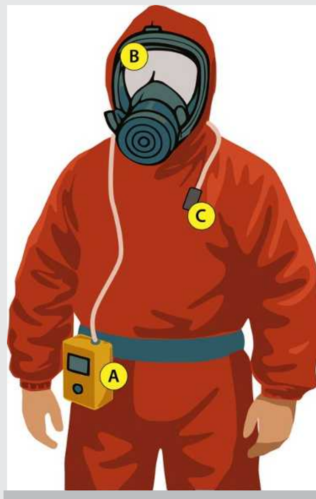
Figure 6-5: Position for personal sampling
