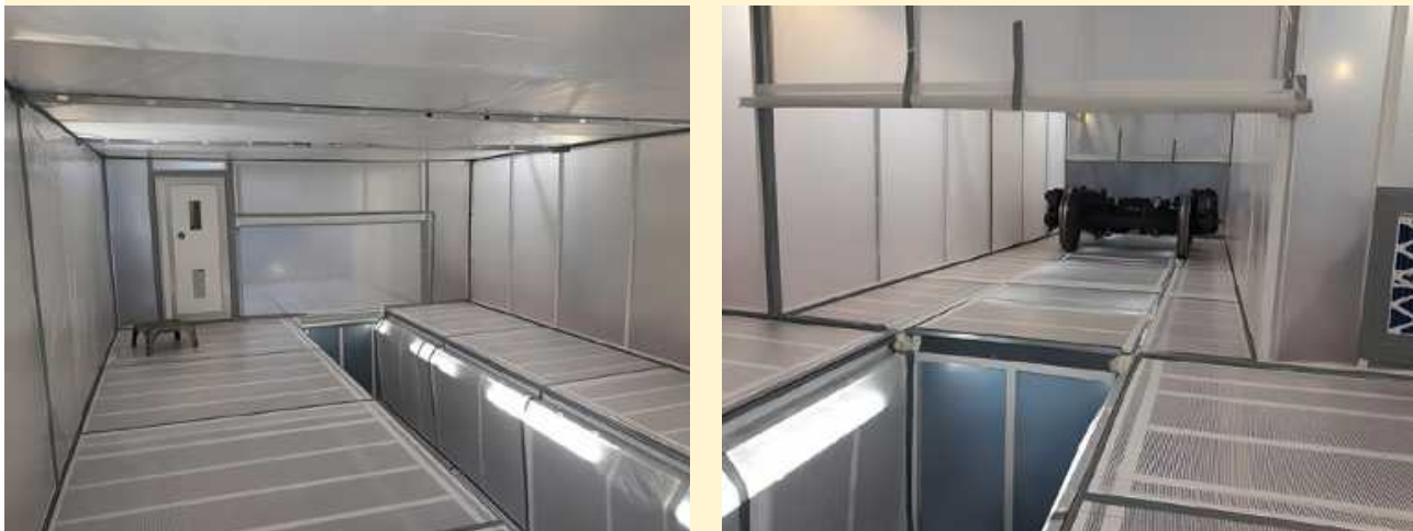
Figure 14-4: Large containment unit with a pit for bogies
